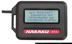
No engine run? check igniton coil check wires to coil Engine Run. All good
